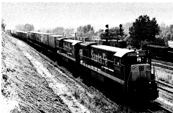
Figure 10: (Left) Santa Fe Railway's new Super C, known as the world's fastest freight train, which goes from Chicago to Los Angeles at top speeds of 79 miles per hour. (Right) British Railways' Freightliner container train, which operates at high speeds throughout the United Kingdom.
